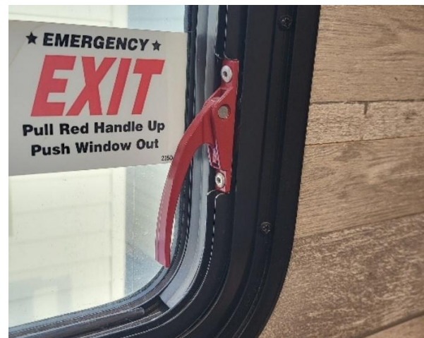
Figure 36. Pull-Lever style latch on an emergency exit. Pull the lever out, away from base, to disengage latch. Push window out.
