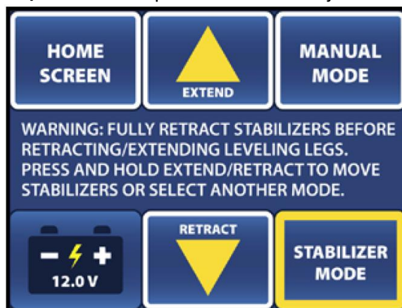
Figure 21. STABILIZER MODE execution screen, allowing manual control of the stabilizers only.
