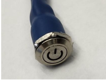
Figure 76. Renogy battery activation cable - power button (switch).
