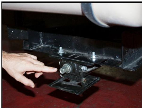
Figure 29. Front stabilizer manual override nut.
