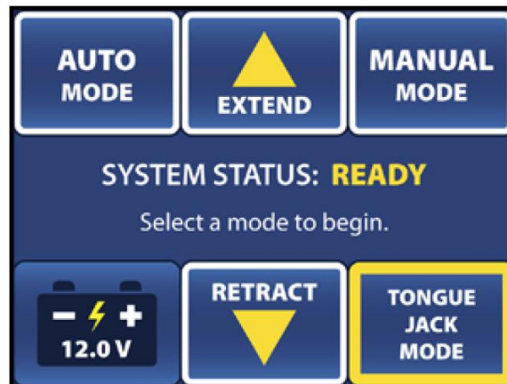
Figure 12. Tongue Jack Mode screen. The yellow highlight indicates the active function.
