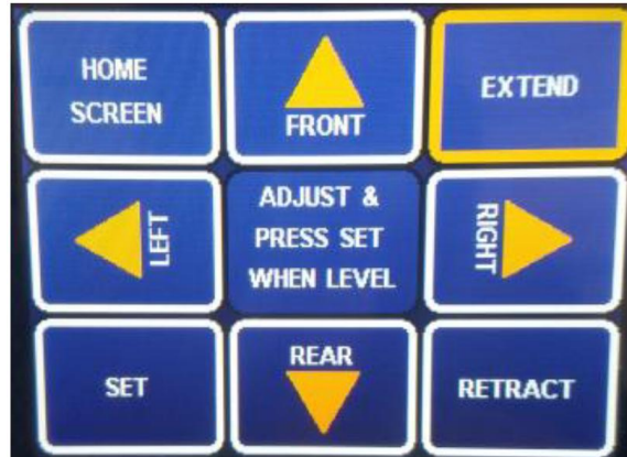
Figure 30. Programming screen of the leveling system.
