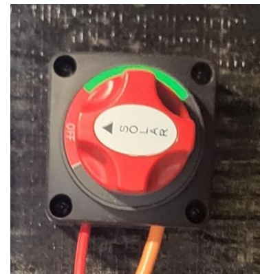
Figure 94. Solar disconnect switch.
