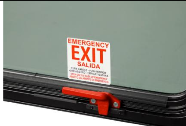
Figure 35. Rotation-Lever style latch on an emergency exit. Rotate the handle up into the window area to disengage the latch. Push window out.
