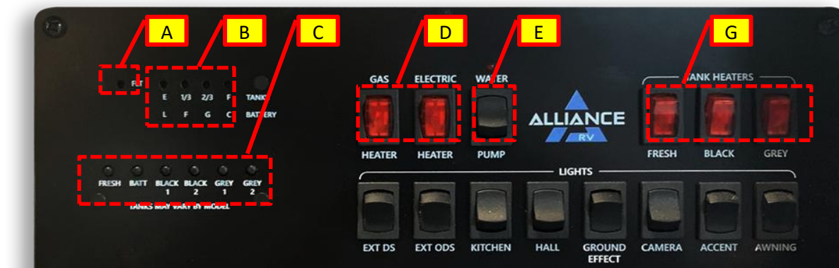
Figure 149. The upper portion of the monitor panel showing tank and water controls. This figure has the same indicators as Figure 122.
