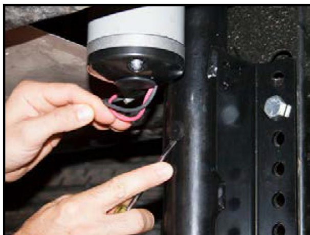
Figure 25. Rear leveling jack grease access hole.
