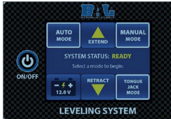
Figure 15. HOME SCREEN display after turning the system on.
