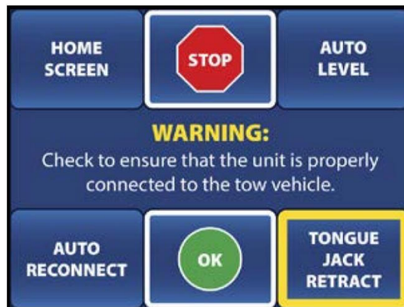
Figure 18. TONGUE JACK RETRACT execution screen.
