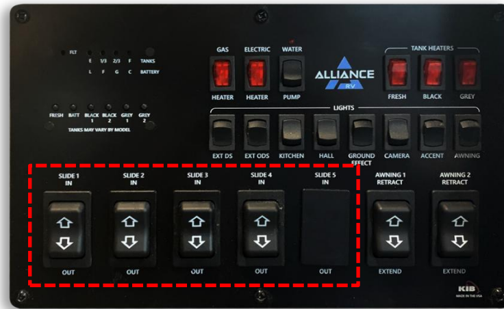
Figure 46. Monitor panel with slide-out controls highlighted.
