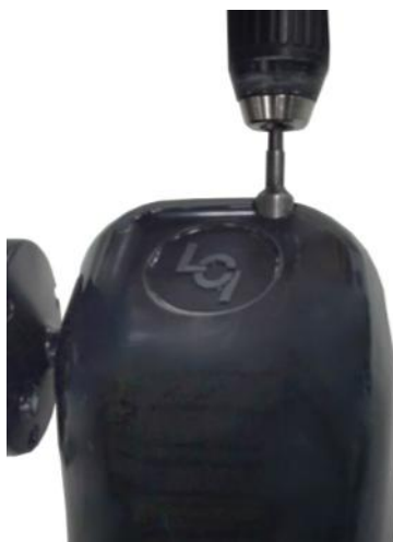
Figure 127. Using a drill to manually retract or extend awning.
