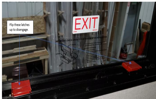
Figure 34. Flip style latch on an emergency exit.
