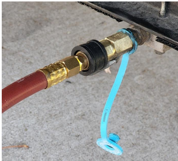
Figure 44. Connected appliance, with flow lever rotated forward to the "on" position.
