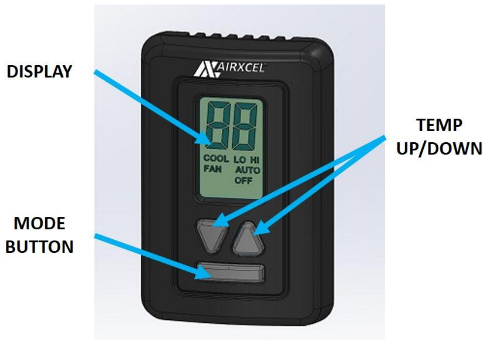
Figure 133. Coleman (Airxcel) LCD Thermostat interface.
