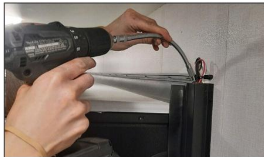
Figure 68. Using the flexible drive tool to manually override the slide.
