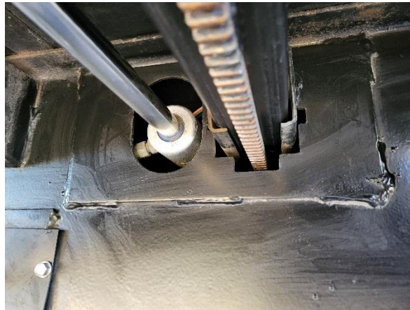
Figure 49. Frame view of the early-model trailers with gear pack inside the frame.
