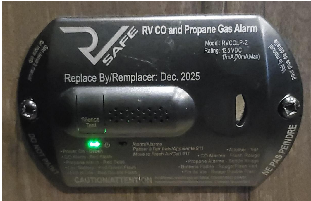
Figure 39. Wall mounted Carbon Monoxide (CO) and Propane alarm. These will be mounted near floor level, usually near stairs.
