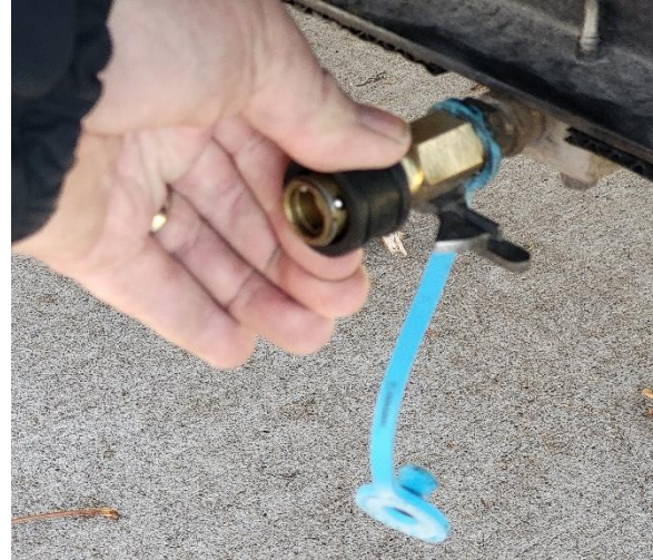
Figure 43. Pushing the retaining ring to accept an appliance connector.
