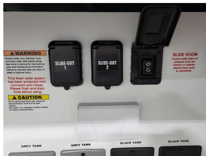
Figure 47. Remote slide controls in the utility bay of the Avenue.
