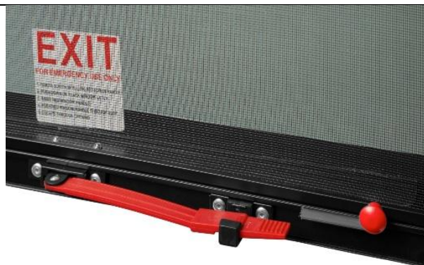
Figure 37. Bar style latch on an emergency exit.
