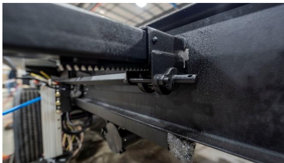
Figure 50. The gear pack is now mounted outside the frame on late-model trailers.
