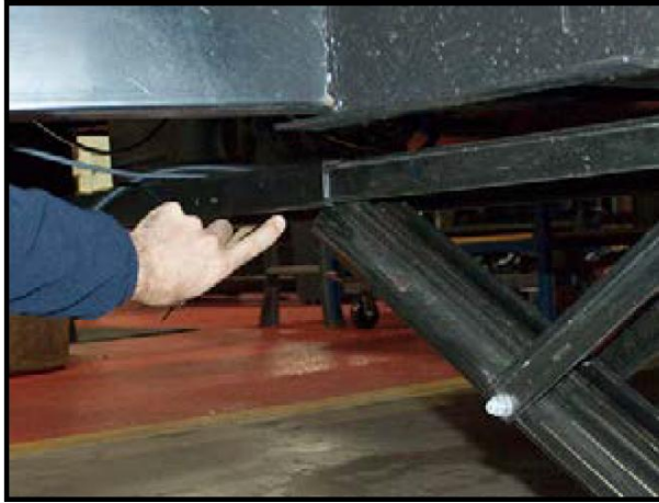
Figure 26. Stabilizer c-jack grease location.
