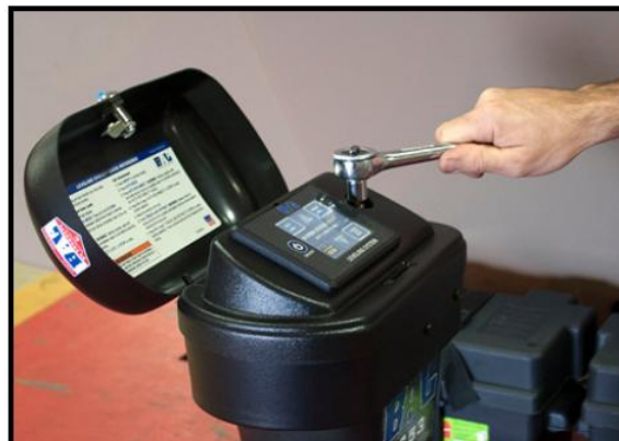
Figure 27. Top of tongue jack manual override.
