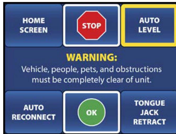
Figure 13. AUTO LEVEL execution screen.
