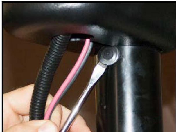
Figure 24. Tongue Jack grease access hole.
