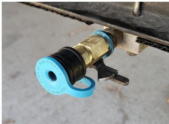
Figure 42. External propane quick connect, with flow lever in the "off" position.
