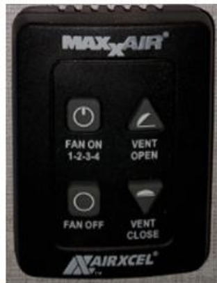
Figure 138. Maxxfan control interface and use. This control is used for the standard (openable) version. The mini has a "Light" button for the upper right button, and motion sensor at the lower right location.
