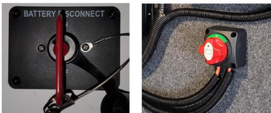
Figure 72. Battery disconnect switches. Original style, left, and new style, right.
