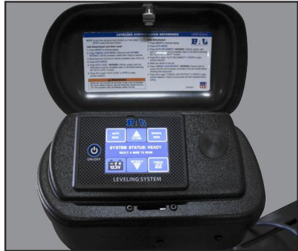
Figure 10. BAL LS 5.3 control display on the tongue jack.
